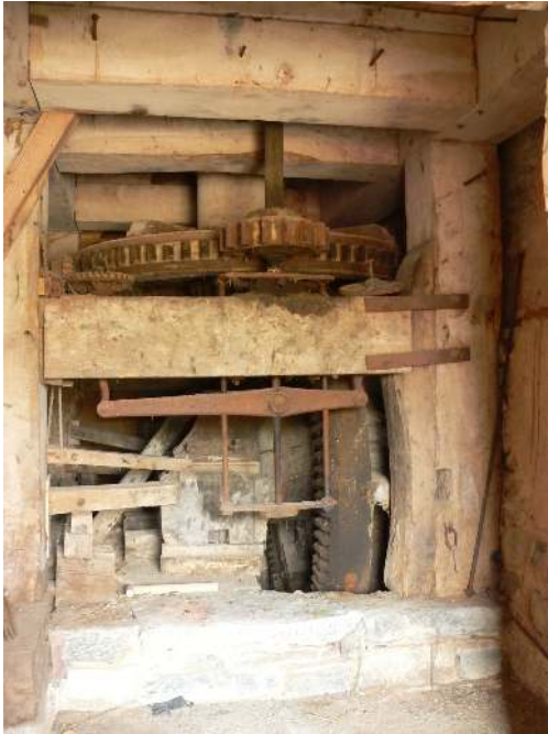
Fig. 15 Stogursey, Castle Street, Town Mill, hurst (photo Martin Watts)
